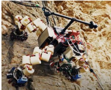
NASA LEMUR robot climbing up a cliff in Titus Canyon and scan for ancient fossils
